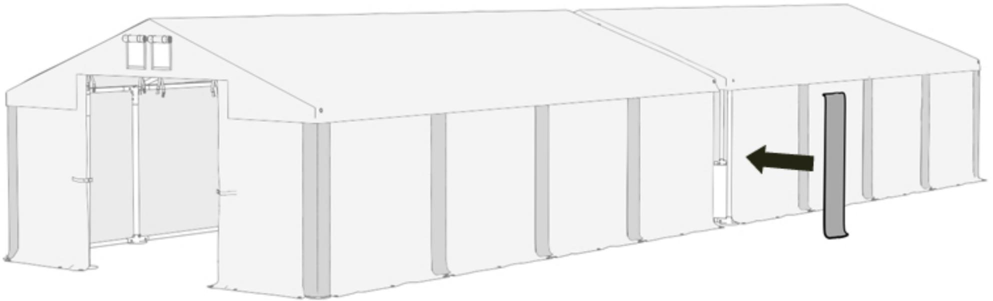
Mount connecting gutter to the roof tarpaulin with the valcros and balls with rubber.
