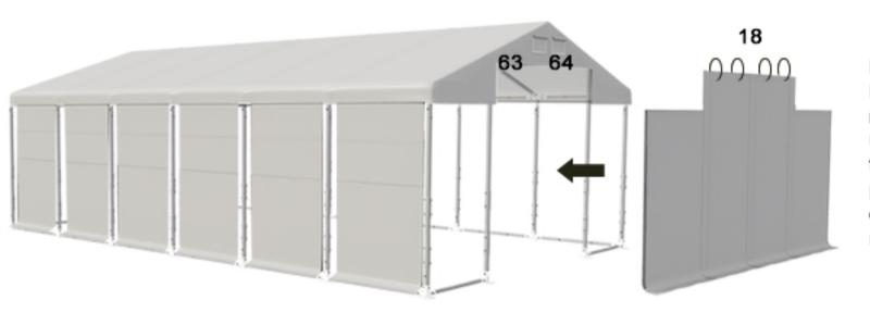
Mount the entrances on the both sides of the tent. Use metal loops (18) to mount the upper part of the entrance to the vertical tube (63 and 64 put together). Sides of the entrance fix using the elastic rubbers with the balls.
