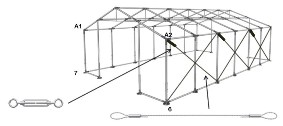
The reinforcement (21) should be connected to the vertical tube (1) and roof tube (61). The reinforcements should be placed on the inside of the tent.
