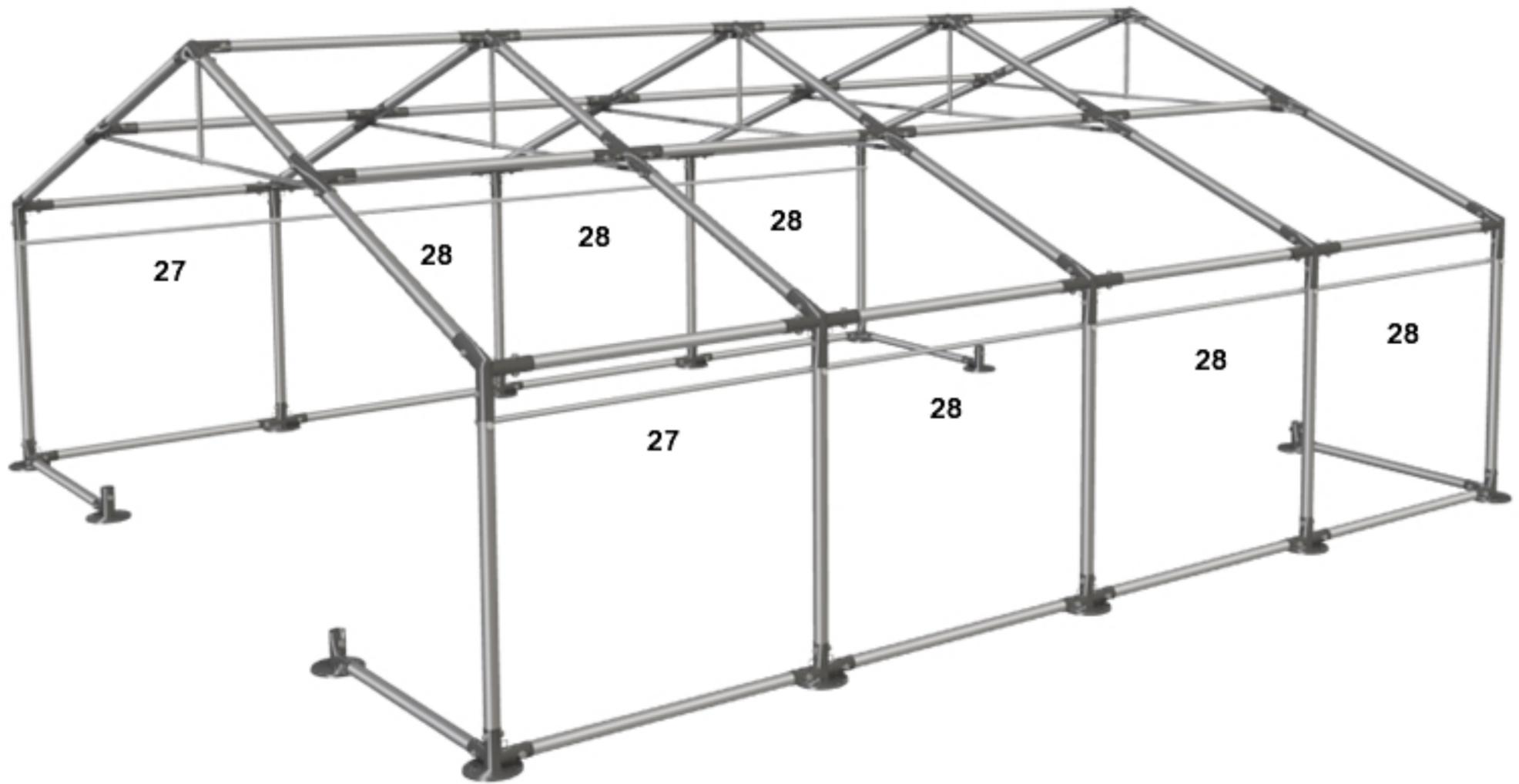
Pass the pipe number 30 through the cover's stitching. Connect pipe (30) with tube (27 or 28), using strings with clips. For tents with the 1m extension, instead of using tube (28) use tube (29). Instead of using tube (30) use tube (31).
