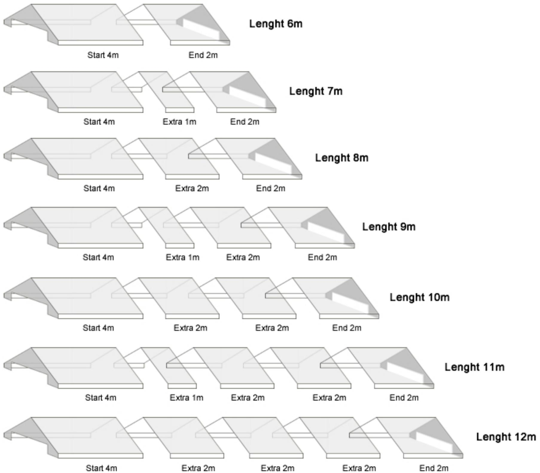
Put the roof cover gently on the construction. Then attach it to the roof frame using elastic rubbers with ball. The elastic rubbers should be installed alternately right - left and front and back.
