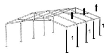
Side panels should be mounted directly to the roof using the velcro stripes. Sides of the panels should be mounted using the elastic rubber with the ball.
