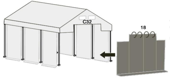
The upper part of the entrance using the metal brackets (18) to the vertical rope (C32). The sides of the entrance should be mounted using the elastic rubber with the ball.
