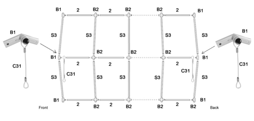
For the tents with the uneven length of the side eg. 9m, 11m, 13m, 21m, 31m.....
