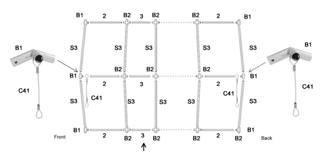
The extension pipe (3) should be located in the second section.
