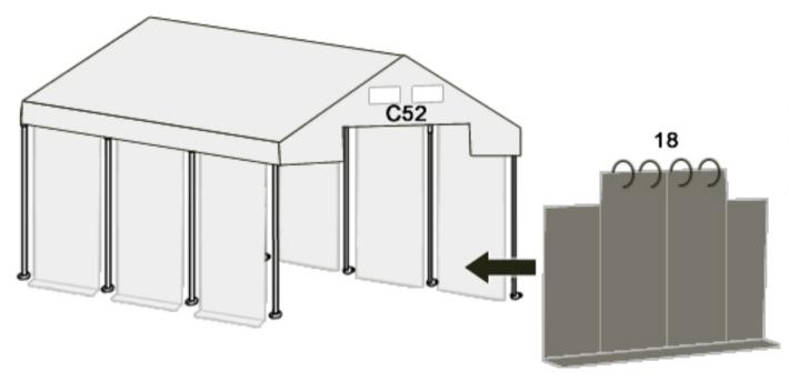
The upper part of the entrance using the metal brackets (18) to the vertical rope (C32). The sides of the entrance should be mounted using the elastic rubber with the ball.
