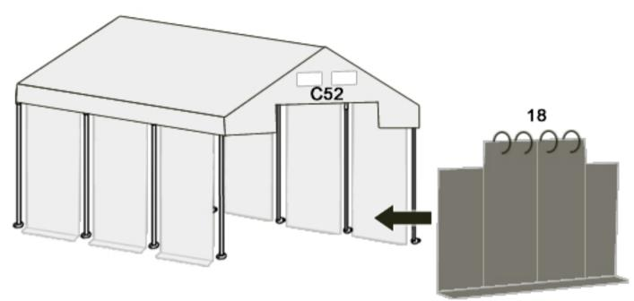
The upper part of the entrance using the metal brackets (18) to the vertical rope (C52). The sides of the entrance should be mounted using the elastic rubber with the ball.
