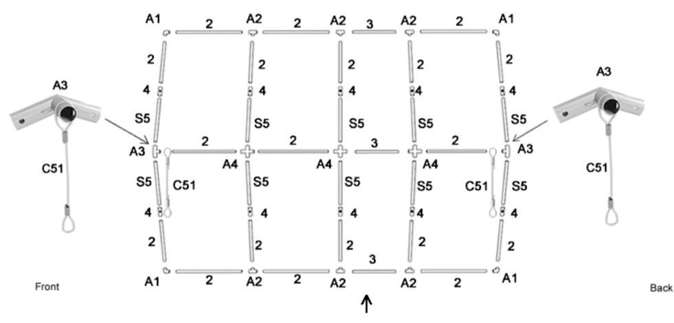
The extension pipe (3) should be located in the third section.
