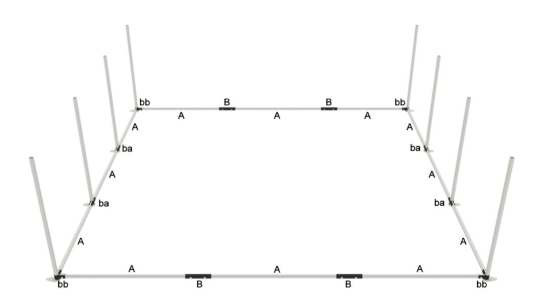
Floor construction should be mounted like it is shown on the picture above. Use S screws.
