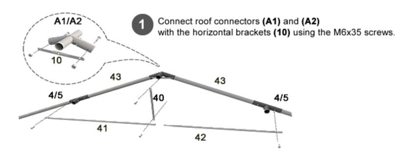
Connect the brackets (41) and (42) using the M6x35 screws. Connect the obtained construction to the lower part of connectors (4 or 5).
