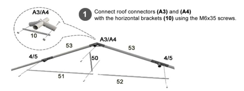
Connect the brackets (51) and (52) using the M6x35 screws. Connect the obtained construction to the lower part of connectors (4 or 5).
