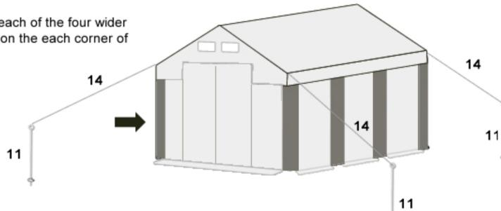
Fix the roof pulls on the corners of the tent using the (14) and (11) parts. All the lines should be tight.
