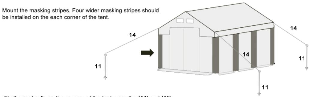
Fix the roof pulls on the corners of the tent using the (14) and (11) parts. All the lines should be tight.
