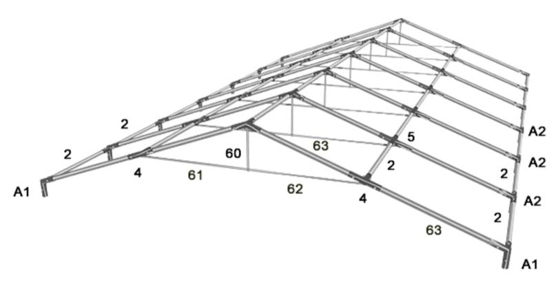
Fully assembled roof construction should look like on the picture above
