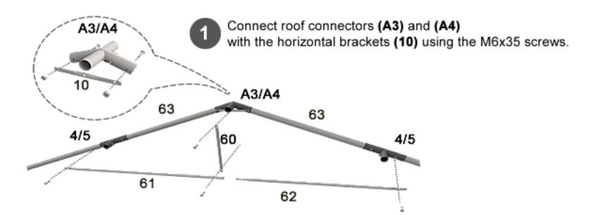
Connect the brackets (61) and (62) using the M6x35 screws. Connect the obtained construction to the lower part of connectors (4 or 5).
